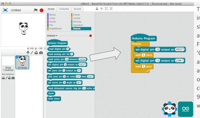
There is an LED light built into your Arduino. This sketch will make it flash on and off a second at a time. From the 'Robots' and 'Control' tabs, drag these actions across and assemble them in this order. You'll need to change the digital pin from 9 to 13 because that's where our LED is.
