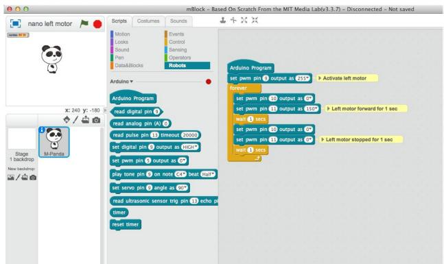
Now repeat the process with the left motor. The left motor is controlled by the pins 9, 10, & 11. Change the pwm pins so your sketch now controls the left motor.
