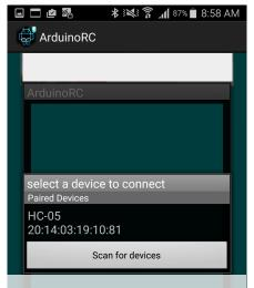
Open the app, confirm your UUID and scan for devices. Look for one called HC-05. Use 1234 for a pairing code if it asks for one. Ensure your robot is powered on.
