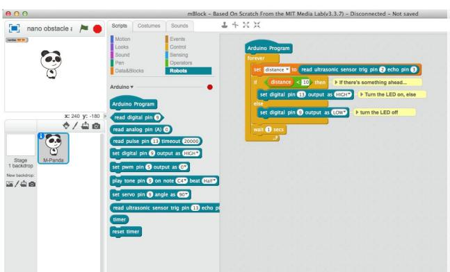
Remember variables from Chapter Two? We're going to use a variable to store the value returned by the ultrasonic sensor. The number will either be high (object is a long way away) or low (the object is close).
